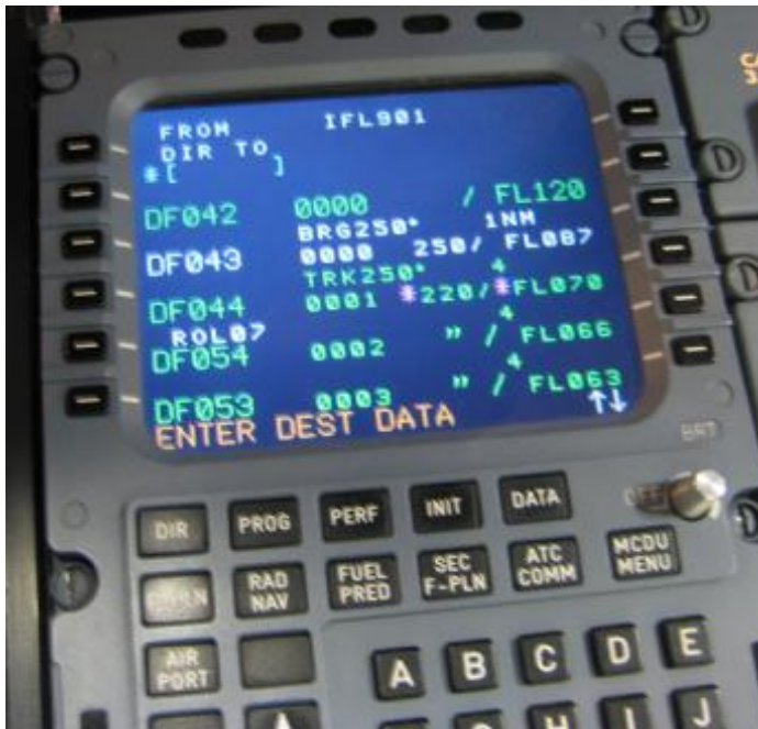
Flight Management System (FMS), Multi-purpose Control and Display Unit (MCDU): screen, line-selector keys and scratch pad - ‚direct‘ key (first row, leftmost key) - waypoint list (on screen)
